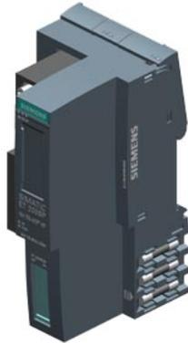
SIPLUS ET 200SP IM155-6DP HF based on 6ES7155-6BA01-0CN0 with conformal coating, -40...+70 °C, bundle PROFIBUS IM, max. 32 I/O modules and 16 ET 200AL modules, multi hot swap, bundle consists of: interface module (6AG1155-6BU01-7CN0), server module (6AG1193-6PA00-7AA0), PROFIBUS plug
