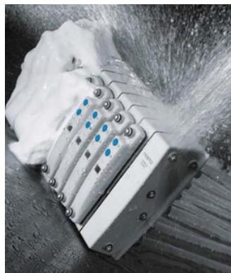
Designed for washdown, the Festo MPA-C valve manifold meets IP69K rating. Note the rounded design which eliminated dead spaces.
