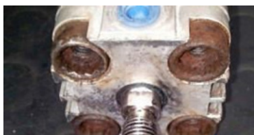
Rusted parts illustrate an incorrect choice of materials.
