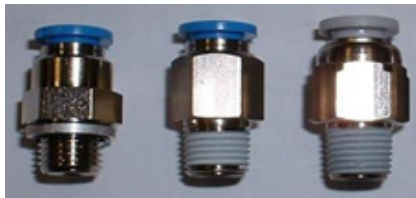
Parallel threads such as G-threads, left, secure to a sealing gasket and eliminate exposed threads. R-threads, center, and NPT, right, require sealing tape and seal by wedging the threads together.
